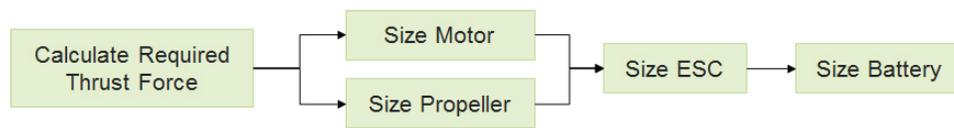
Note: The motor and propeller must be sized *together* as it is the combination of the two that produces the thrust force (more on this below). The motor/propeller is the challenging part—once selected, the ESC and battery are simple to choose.
